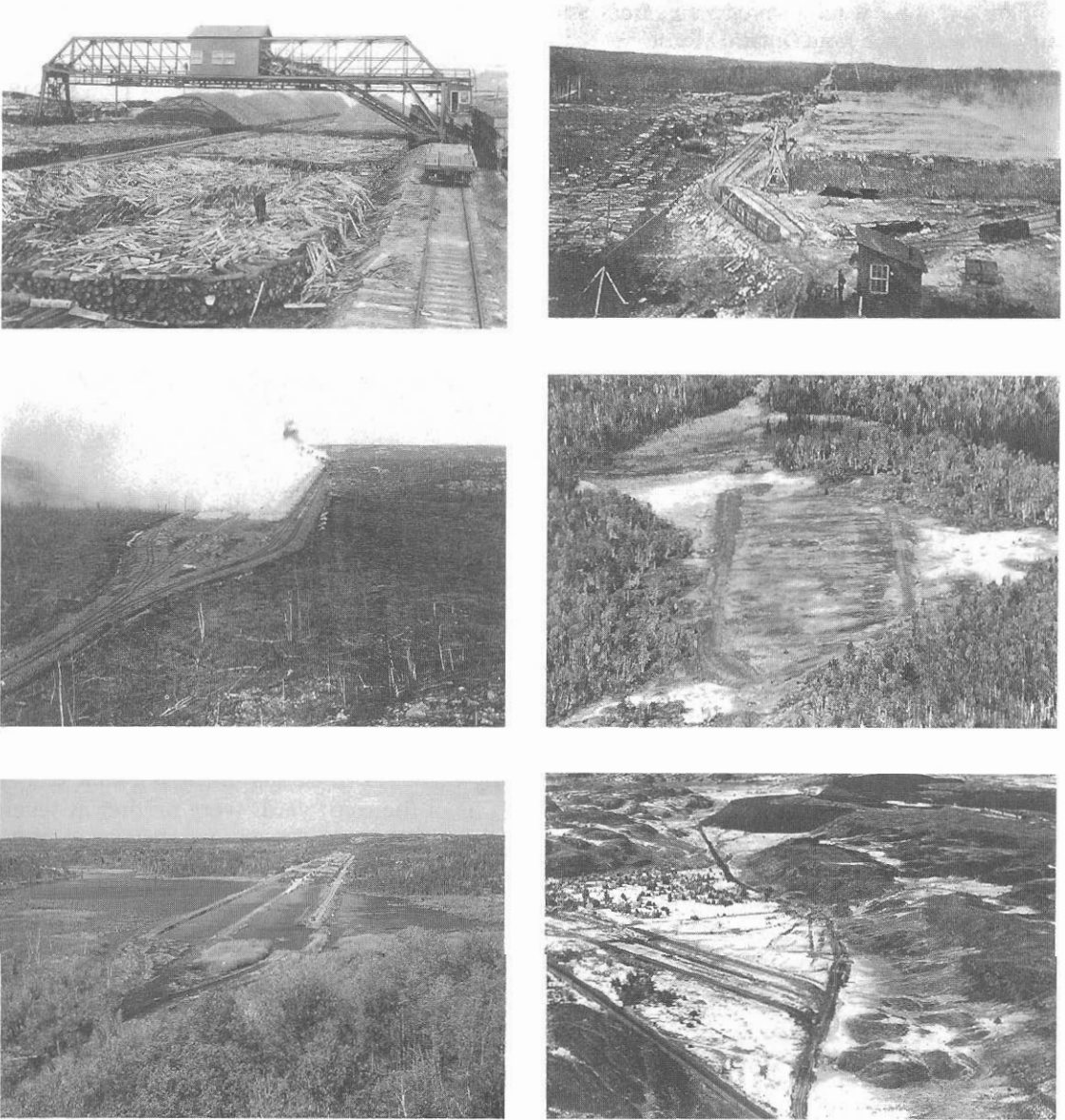
FIGURE 2.5. Roast yards in the Sudbury area. ( Upper left ) A 1920 view of the O'Donnell roast yard, showing wood and ore piled before ignition. The O'Donnell ( center left ) and circa 1901 Victoria Mine ( upper right ) roast yards during the roasting process. The Victoria Mine roast yard in 1979 ( center right ) and the O'Donnell yard in 1994 ( lower left ), showing the recovery of vegetation to the edge. ( Lower right ) A 1979 picture of the Coniston roastbed, that operated from 1913 to 1918, set in a landscape that is still almost completely barren. (Photos courtesy of Inco Archives, W. McIlveen and E. Snucins.)
